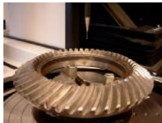
Measurement of bevel gears
